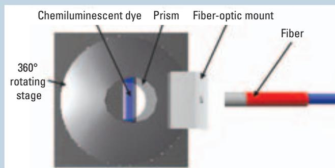
Top view of the experimental geometry and major components used for SPCC.
