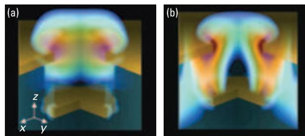
(a) Computed electromagnetic field distribution associated with resonance at 883 nm shows that the intensity is concentrated at the edges of the nanoholes in the upper level of the crystal. (b) The distribution with resonance at 1138 nm displays strong coupling between the upper and lower levels of the crystal. (Adapted with permission. Copyright 2006 National Academy of Sciences, U.S.A.)
