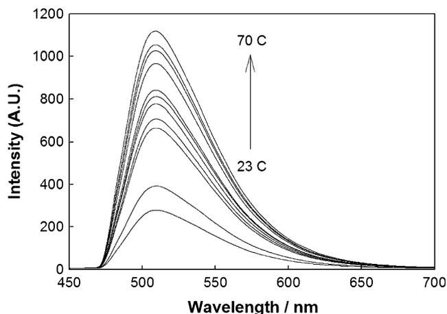
Fig. 5. Emission spectra of acridine yellow, AY ( $\lambda_{ex} = 473$  nm) in bulk solution as a function of temperature (heated with Peltier system).
