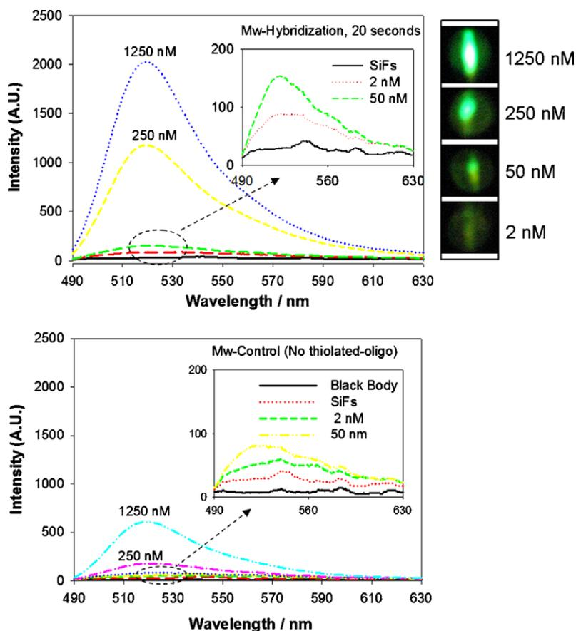
Fig. 3. Emission spectra of Fluorescein-Oligo as a function of concentration after 20 s low power microwave heating (top); photographs showing an increased emission intensity as a function of FI-DNA concentration after 20 s Mw heating. Bottom—A control sample identical to the top panel but with no surface bound SH-Oligo anchor.
