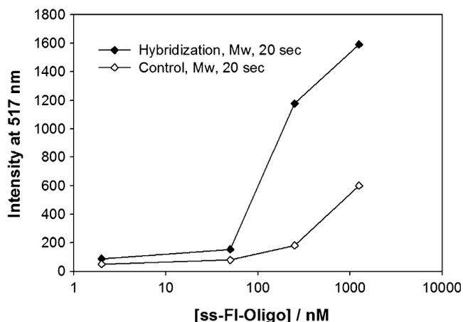
Fig. 4. Semi-logarithmic plot of the fluorescence emission intensity at 517 nm for the Fluorescein-Oligo as a function of concentration derived from Fig. 3.
