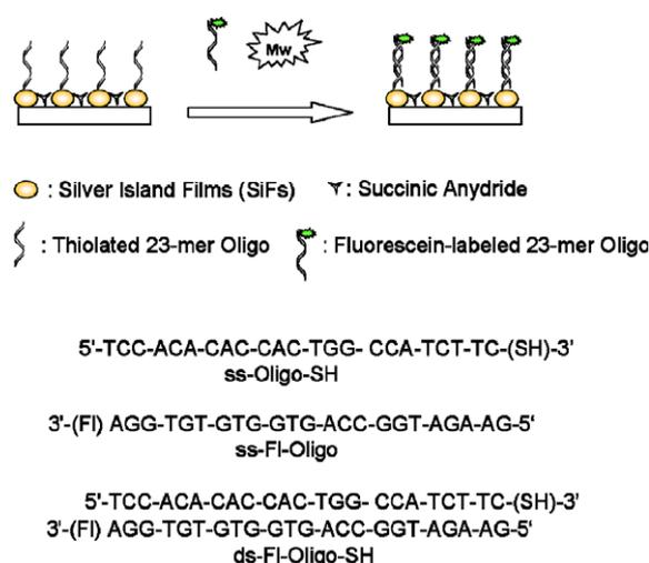
Fig. 1. Microwave-accelerated metal-enhanced fluorescence-based sensing scheme for fast and sensitive DNA target detection. The lower panel shows the structures of the DNA oligomers used in this study.
