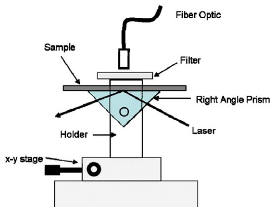
Fig. 2. Total-internal reflection fluorescence (TIRF) geometry for DNA hybridization assays.
