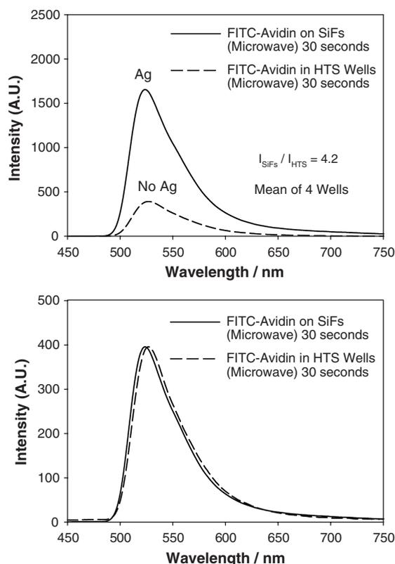
Fig. 5. Fluorescence emission intensity of fluorescein from both silvered and non-silvered HTS wells (Top) after 30 s microwave heating. The spectra are the average of 4 wells. (Bottom) Normalized spectra from both silvered and non-silvered wells after microwave heating.
