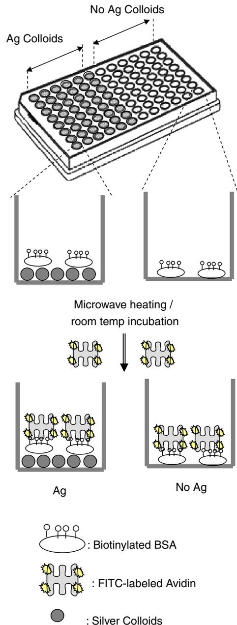
Fig. 2. Sample geometry in HTS wells.
