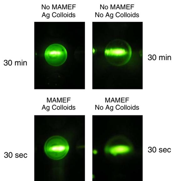
Fig. 6. Photographs of actual HTS wells, with and without silver, before and after microwave heating. The photographs were taken through a long-pass filter with 473 nm TIR evanescent wave excitation.
