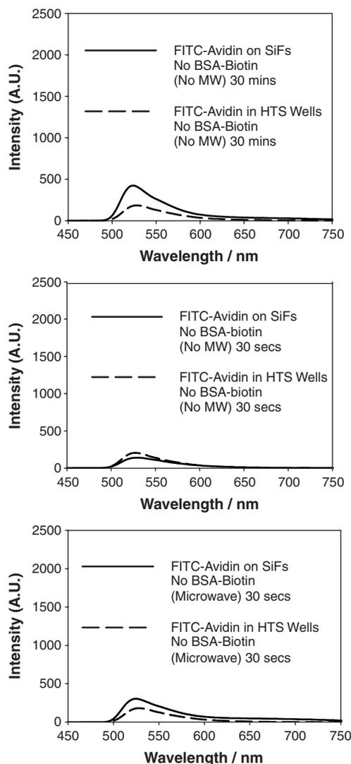
Fig. 7. Control experiments showing the rate of non-specific absorption of fluorescein–avidin to bare and silvered surfaces after 30 min incubation (Top), 30 s incubation (Middle), and after 30 s low power microwave heating (Bottom). The well bottoms were not coated with Biotinylated-BSA.
