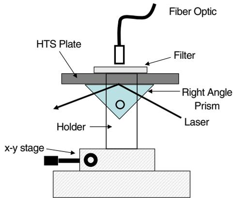
Fig. 1. TIRF—Total Internal Reflection Fluorescence experimental set-up mounted on an XY stage, for analysis of both the silvered and unsilvered HTS wells.
