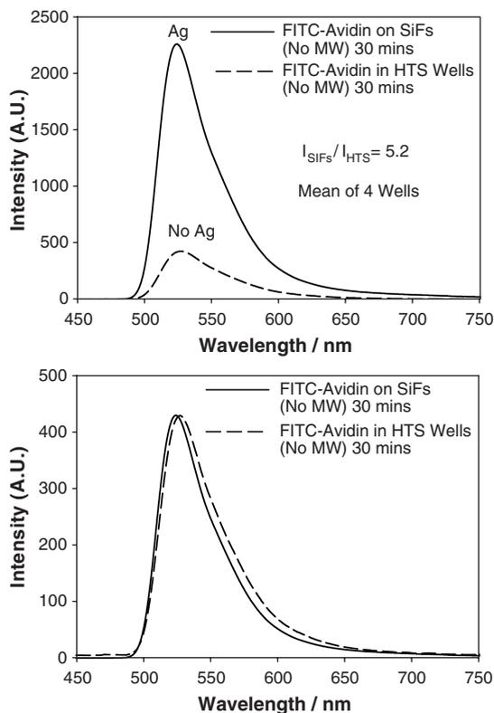
Fig. 4. Fluorescence emission intensity of fluorescein from both silvered and non-silvered HTS wells (Top) after 30 min room temperature incubation. The spectra are the average of 4 wells. (Bottom) Normalized spectra from both silvered and non-silvered wells.
