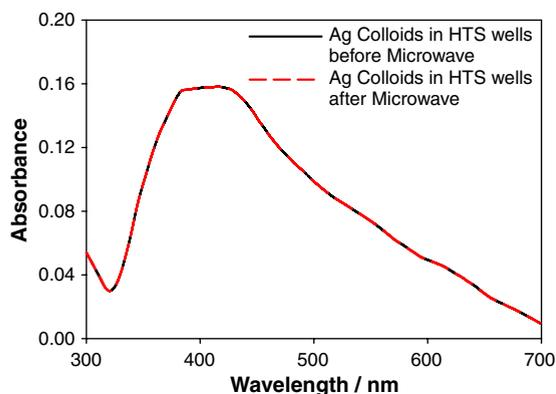
Fig. 3. Absorption spectra of silver-colloid coated plastic-bottomed HTS wells, before and after low power microwave heating.
