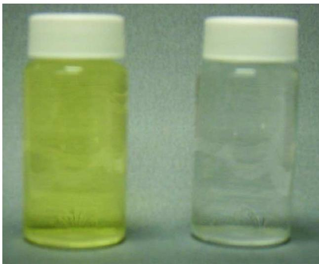
Fig. 5. Photograph of two vials containing equal concentrations of BAQBA and both 0 and 300 mM fluoride, left and right, respectively.
