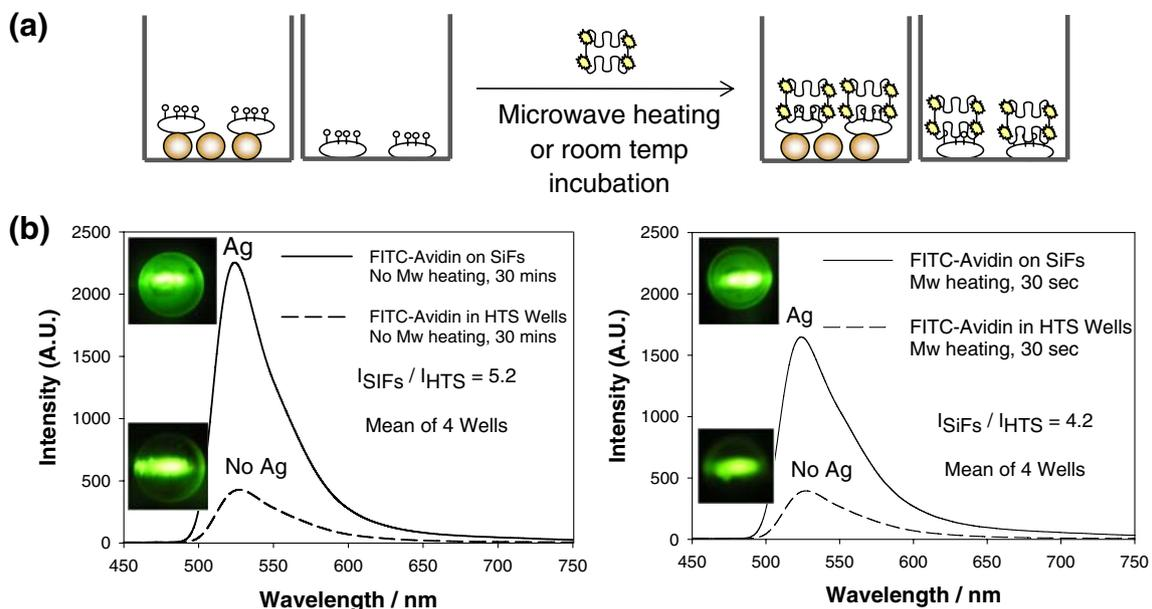
**Fig. 6** A model MAMEF-based protein detection assay for HTS wells. **a** Model protein-fluorophore system used to demonstrate MAMEF in HTS wells; **b** emission spectra of FITC for a model protein assay run at
