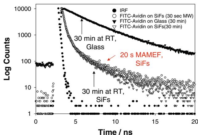
**Fig. 5** Fluorescence lifetime studies for the fluorophore used in the MAMEF-based protein detection assay. Intensity decays for fluorescein isothiocyanate (FITC)-Avidin on both glass and SiFs, both before and after exposure to low power microwave heating. The intensity decays on the SiFs are almost identical. IRF, instrument response function. Adapted from [1]
