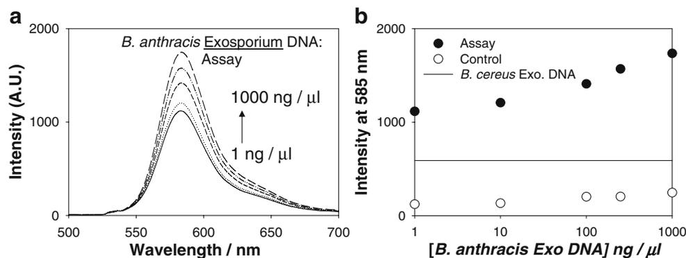
**Fig. 11** MAMEF-based anthrax DNA hybridization assay on Silvered glass substrates. **a** Emission spectra of the TAMRA-Oligo as a function of *B. anthracis* exosporium concentration after 30 s of low-power micro-
