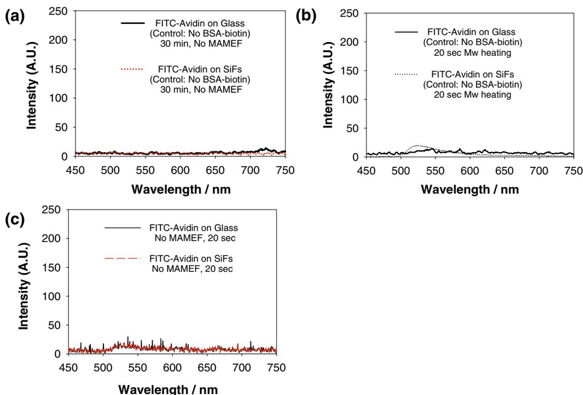
**Fig. 4** Control experiments for the model MAMEF-based protein detection assay. **a** Control experiment, where one of the protein binding partners, BSA-biotin, is omitted from the assay, run at room
