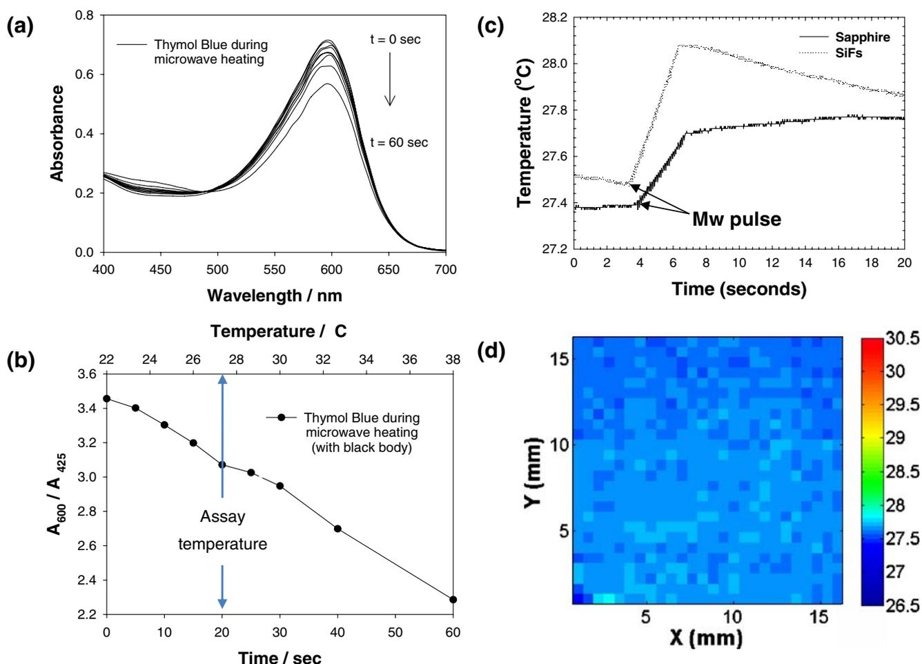
**Fig. 2** Real-time monitoring of temperature changes during microwave heating. **a** Absorption spectra as a function of temperature for 30  $\mu$ l thymol blue measured during microwave heating; **b** the respective absorbance, temperature vs time ratiometric plot; **c** real-
