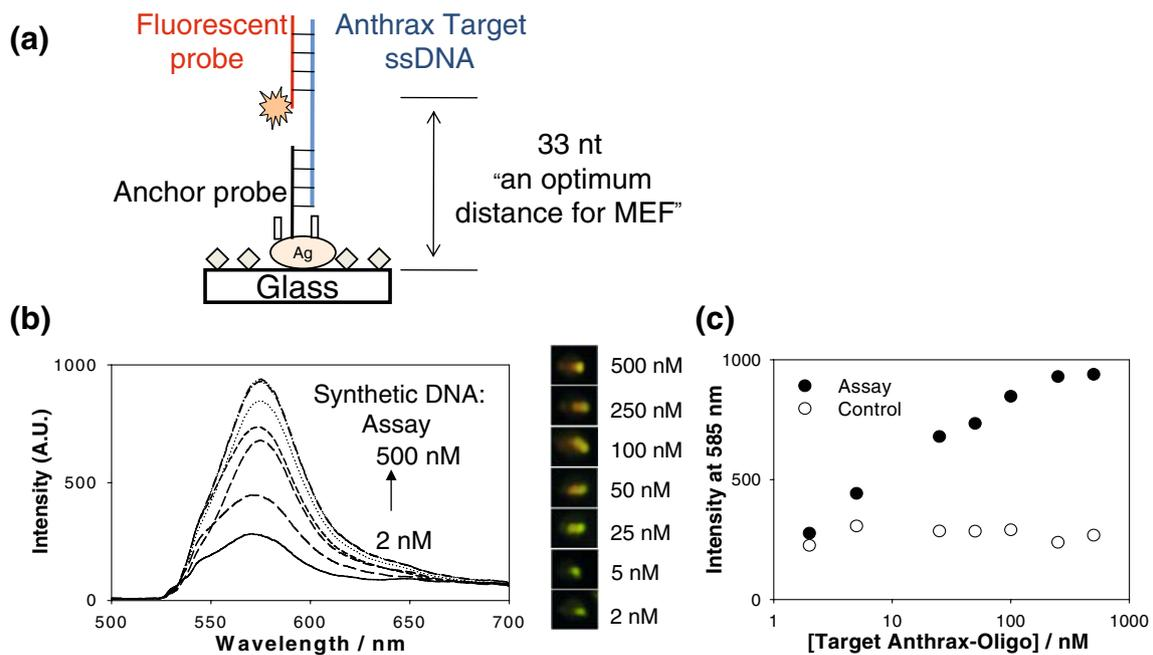
**Fig. 10** MAMEF-based anthrax DNA hybridization assay on silvered glass substrates. **a** Experimental design, depicting the organization of the DNA oligomers on SiFs used for the detection of *B. anthracis*. **b** Emission spectra of TAMRA-ssDNA as a function of concentration after 30 s of low-power microwave heating. Photographs showing the
