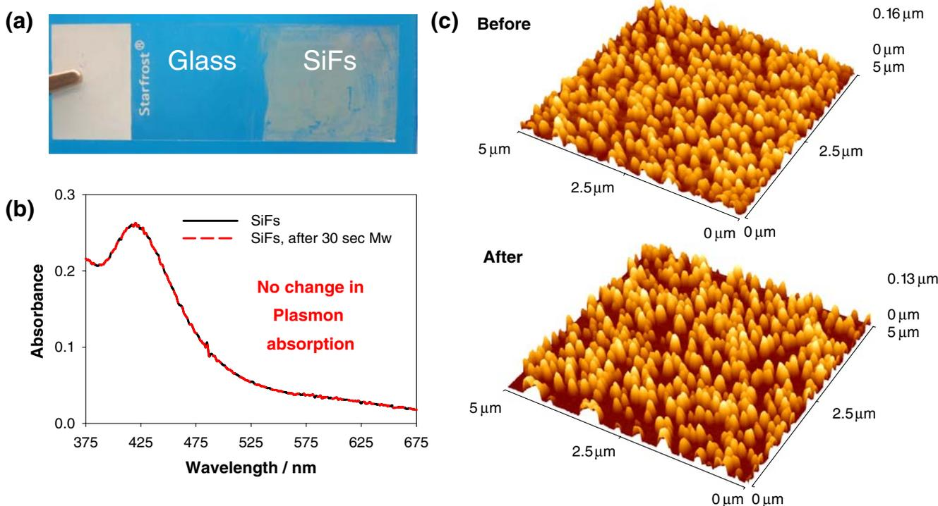
**Fig. 1** Sample characterization studies. **a** A typical photograph of silver island films (SiFs) deposited glass substrate, **b** plasmon absorption spectra both before and after microwave heating, and **c** the corresponding AFM images. Adapted from [1]
