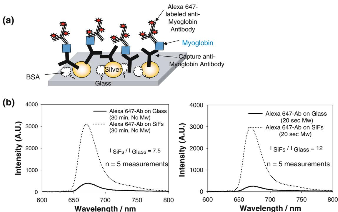
**Fig. 7** MAMEF-based myoglobin detection assay on glass substrates. **a** Myoglobin immunoassay; **b** fluorescence emission spectra of Alexa-647 for the myoglobin immunoassay on SiFs-deposited glass substrates after
