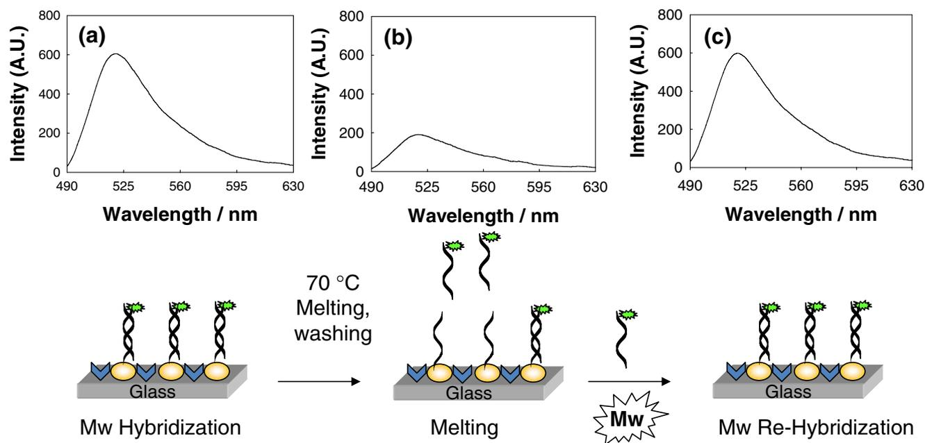
**Fig. 9** Reversibility of the model DNA hybridization assay on glass substrates. Emission spectra of fluorescein-DNA **a** after hybridization, **b** after melting at 70°C, and **c** after a further 20-s low-power microwave
