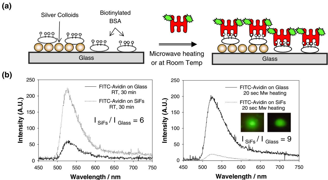
**Fig. 3** A model MAMEF-based protein detection assay. **a** Model protein-fluorophore system used to demonstrate MAMEF on glass substrates; **b** emission spectra of fluorescein isothiocyanate (FITC) for
