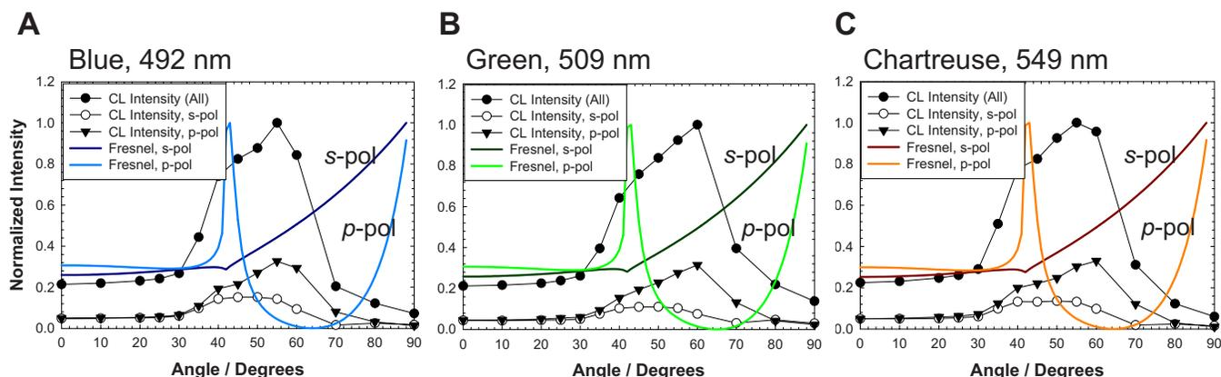
FIG. 4. (Color online) Normalized intensity curves of chemiluminescence emission, *s*-polarized emission, and *p*-polarized emission from  $100 \mu\text{l}$  of dye on 15 nm iron thin films as compared with the theoretical Fresnel curves for (a) blue at 492 nm, (b) green at 509 nm, and (c) chartreuse at 549 nm.
