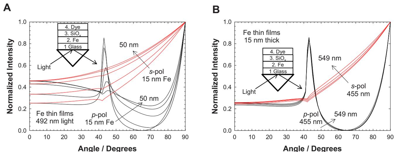
FIG. 2. (Color online) (a) Four-phase Fresnel reflectivity curves for *p*- and *s*-polarized lights at 492 nm for iron thin film thicknesses of 15, 20, 30, 40, and 50 nm with a 10 nm SiO<sub>x</sub> overlayer. (b) Four-phase Fresnel reflectivity curves for *p*- and *s*-polarized lights at 455, 492, 509, and 549 nm for 15 nm iron thin films with a 10 nm SiO<sub>x</sub> overlayer.
