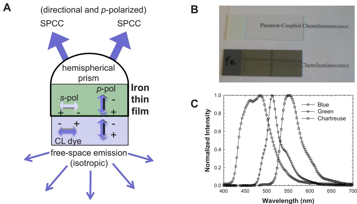
FIG. 1. (Color online) (a) Schematic depiction of SPCC from iron thin films. (b) Photographs of 15 nm iron thin films as compared to a blank glass slide. The printed text “Plasmon-Coupled Chemiluminescence” below the slides demonstrates the semitransparent nature of the films. (c) Normalized spectra of blue, green, and chartreuse emissions. CL: chemiluminescent.
