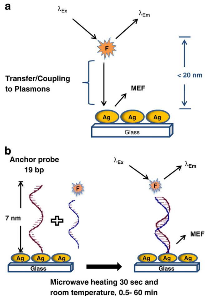
**Fig. 1.** (a) Graphical representation of the current interpretation of MEF. (b) MAMEF surface DNA capture assay, annealing in microwave cavity and the control assay run at room temperature, "Rapid Catch and Signal" technology.
