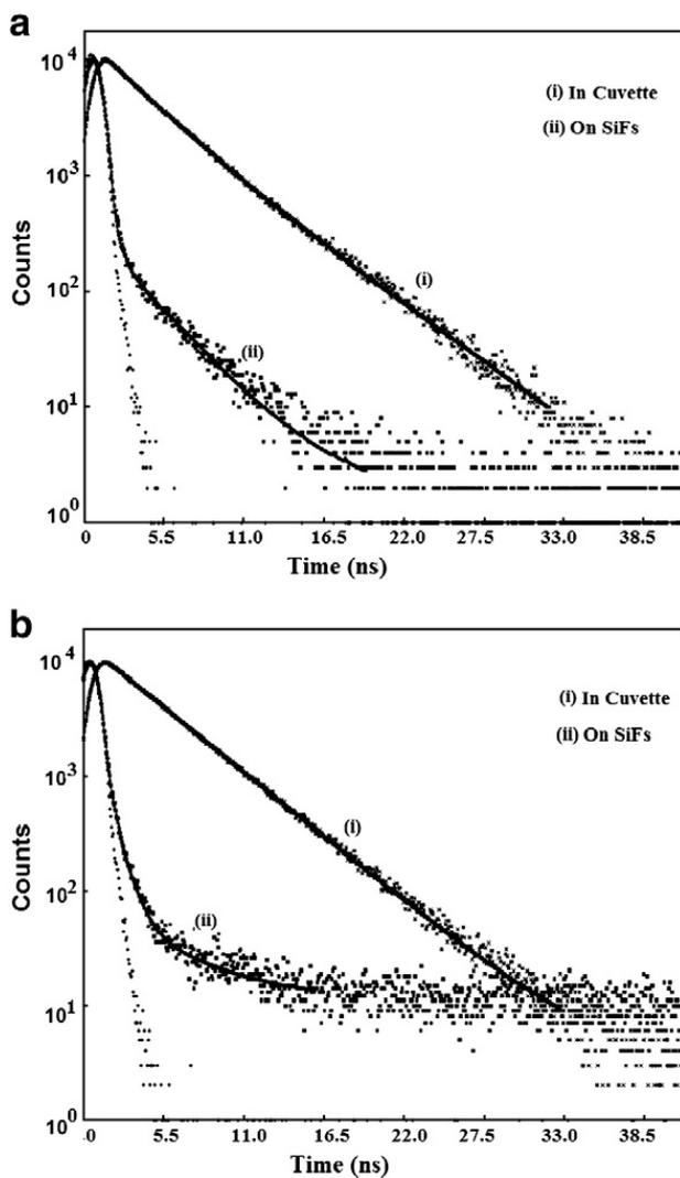
Fig. 4. Intensity decay profile of (a) Alexa 488 and (b) Alexa 594 on glass, a SiFs sandwich and in solution (cuvette)  $\lambda_{ex} = 467$  nm.
