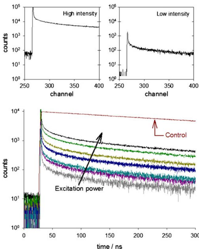
**Fig. 2** The lower panel shows time-resolved fluorescence decay curves recorded for a range of different excitation powers of a Ruthenium dye on a SiF surface. The excitation wavelength was 474 nm and the emission was collected through a RazorEdge 488 nm filter combined with longpass filters centred at 550 nm and 590 nm. The upper panel shows decay curves recorded at an excitation power of 32.6  $\mu\text{W}$  (high intensity) and at 0.03  $\mu\text{W}$  low intensity
