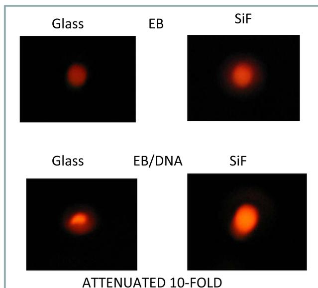
**Fig. 4.** Digital photographs of the fluorescence spots of free EB and EB in complex with 16 bp DNA, loaded on SiFs and glass slides. Attenuation of EB/DNA emission was undertaken using a neutral density filter for emission (OD = 1.0), attenuation was 10-fold. Power of a 473 nm laser was 500 mW. The ratio of EB/DNA = 1:1, [DNA] = 4  $\mu$ M.
