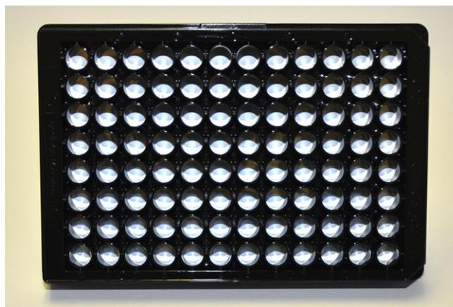
Fig. 1. Photograph of silvered 96-well plates, or Quanta Plates™, used for assay development.
