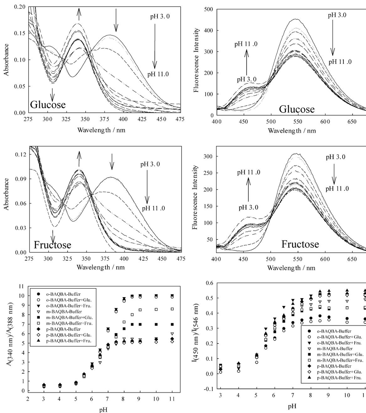
Fig. 6. Absorption and fluorescence emission ( $\lambda_{\text{ex}} = 358 \text{ nm}$ ) for *m*-BAQBA in the presence of glucose, top, fructose, middle, and the respective ratiometric plots for all three isomers both with and without sugars, bottom panels.
