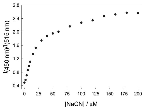
Fig. 2. Fluorescence emission spectra of DSTBA with increasing concentrations of aqueous cyanide (top) and the respective ratiometric plot using the intensities at 450 and 515 nm (bottom).
