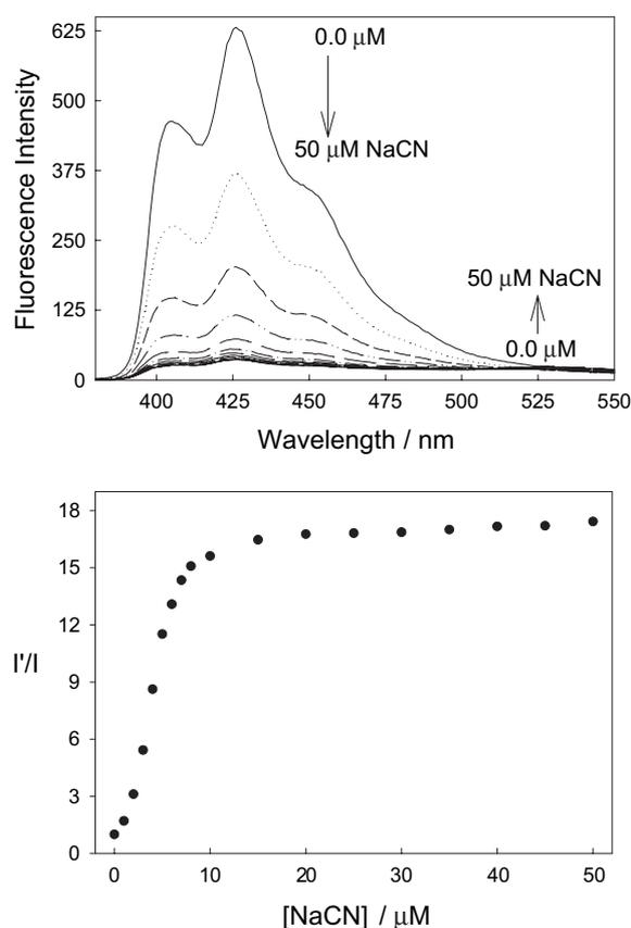
Fig. 5. Fluorescence emission spectra of ANDBA with increasing concentrations of aqueous cyanide (top) and the respective ratiometric type plot using the initial fluorescence intensity,  $I'$ , at 425 nm in the absence of cyanide, and in the presence of increasing cyanide concentrations,  $I$  (bottom).
