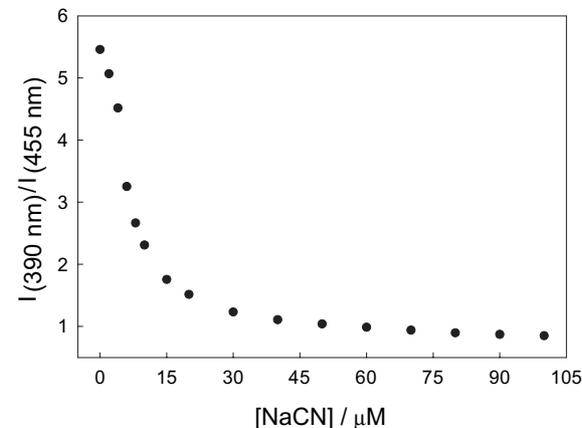
Fig. 3. Fluorescence emission spectra of CSTBA with increasing concentrations of aqueous cyanide (top), and the respective ratiometric plot using the intensities at 390 and 455 nm (bottom).
