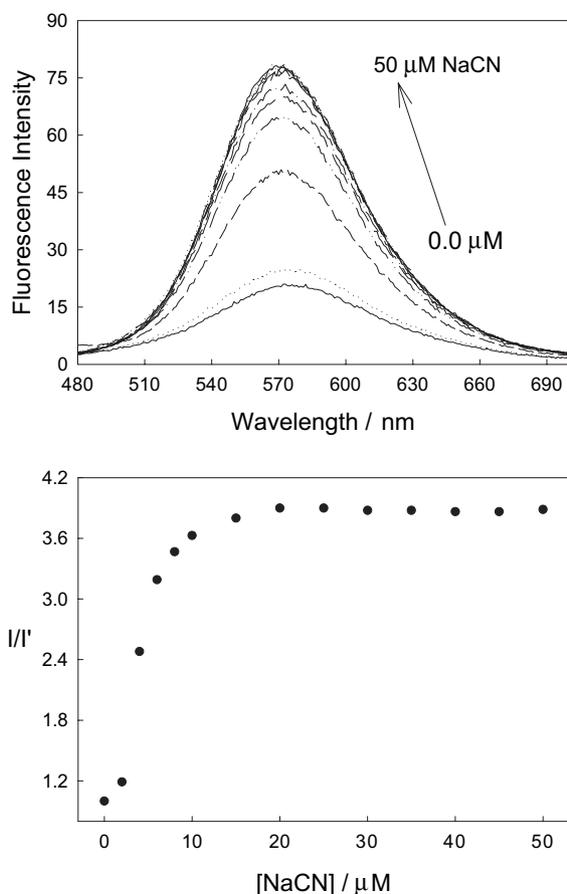
Fig. 4. Fluorescence emission spectra of Chalc 1 with increasing concentrations of aqueous cyanide (top), and the respective ratiometric type plot using the initial fluorescence intensity,  $I'$ , at 570 nm in the absence of cyanide, and in the presence of increasing cyanide concentrations,  $I$  (bottom).
