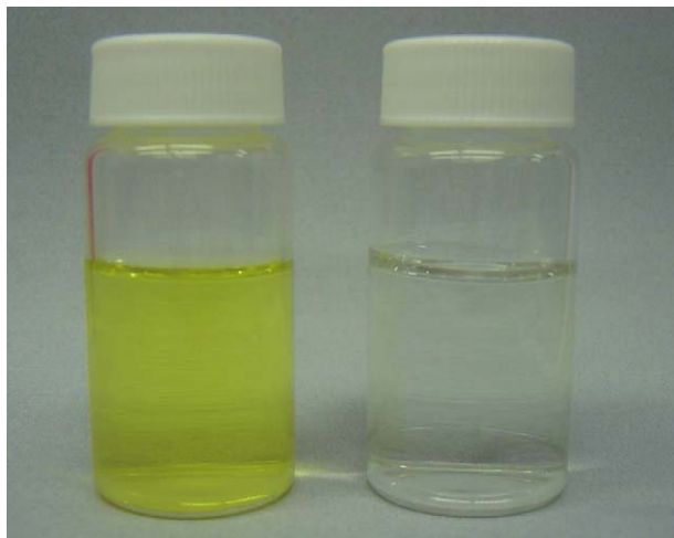
Fig. 5. Photograph of two vials containing equal concentrations of o -BAQBA and both 0 and 10 \mu\text{M} NaCN, left and right, respectively. Very similar findings were observed for all three boronic acid probes.
