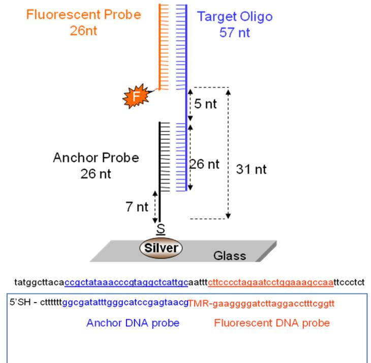
**Figure 4.** (Top) MAMEF assay construction for Chlamydia DNA. The anchor DNA probe, target DNA and fluorophore DNA probe, (Bottom).
