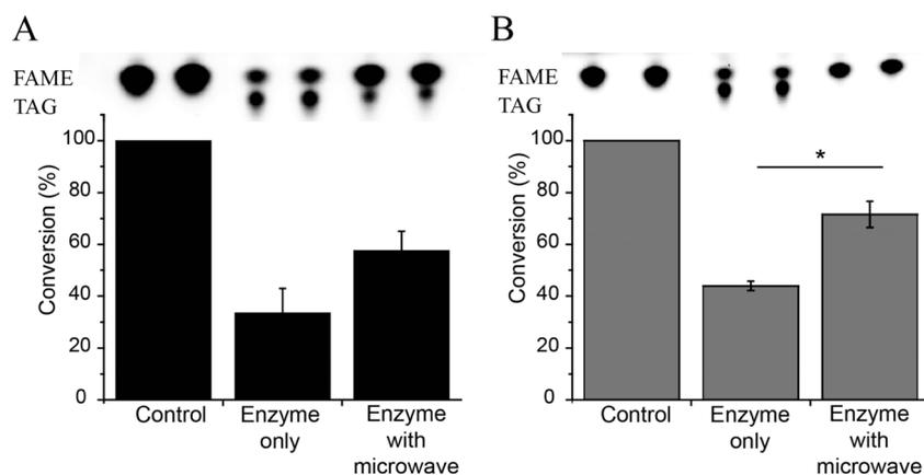
**Fig. 6** Effect of microwave pretreatment on in situ enzymatic conversion from *Scenedesmus* sp. HTB1 biomass. **a** Comparison of the FAME yield using HTB1 biomass with and without a 30% power (270 W) microwave pretreatment prior to in situ enzymatic conversion reaction. **b** Comparison of the yield using HTB1 biomass with and without a 40% power (360 W) microwave pretreatment prior to in situ enzymatic conversion reaction.
