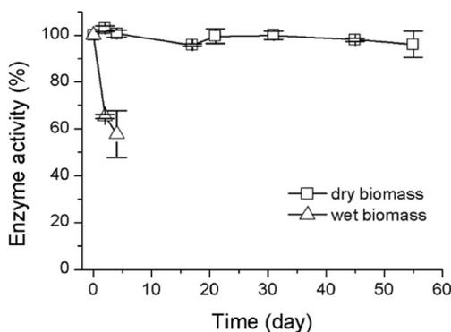
**Fig. 5** Enzyme stability under optimized reaction conditions for wet (open triangle) or dry algae biomass (open square). Reaction conditions were wet biomass to *t*-butanol to methanol weight ratio of 1:1:2 at 45 °C or dry biomass to *t*-butanol to methanol weight ratio of 1:2:0.5 at 25 °C. Data represented mean ± SD of triplicate experiments
